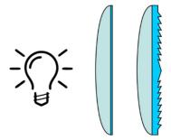
Figure 13. Lens orientation
