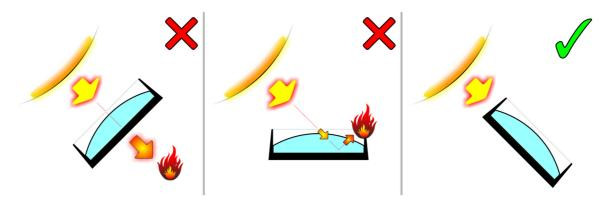
Figure 1. Avoiding damage from light sources
