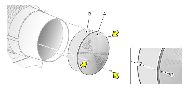
Figure 12. Removing a micro-Fresnel lens
