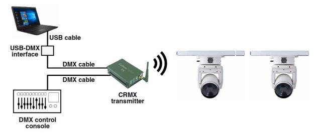
Figure 10. CRMX wireless control system
