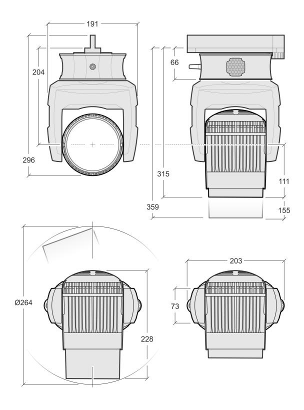
Dimensions given in millimeters
