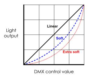
Figure 3. Dimming curves
