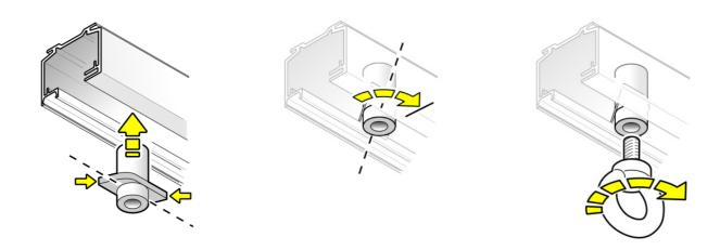
Figure 8. Installing a retaining collar and safety cable
