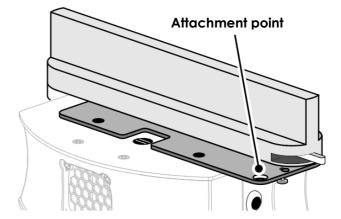
Figure 7. Safety cable attachment point
