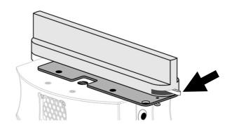
Figure 5. Main mechanical fastener lever
