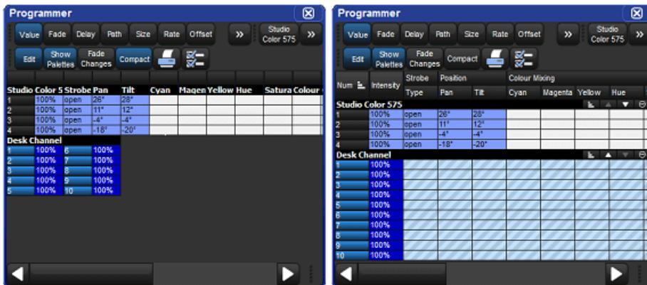
Figure 2.7. A spreadsheet with and without Compact Mode
