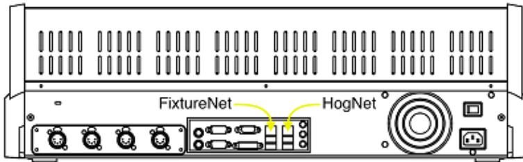
Figure 3.6. HogNet and FixtureNet Connections on back panel of Road Hog 4 Console
