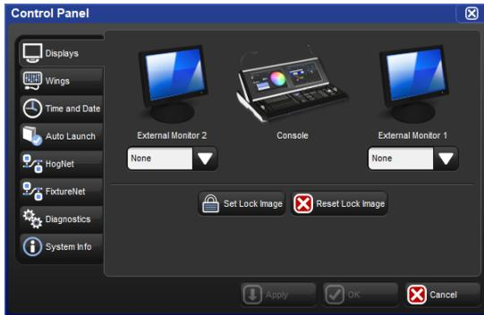
Figure 30.1. The Displays pane of the Control Panel
