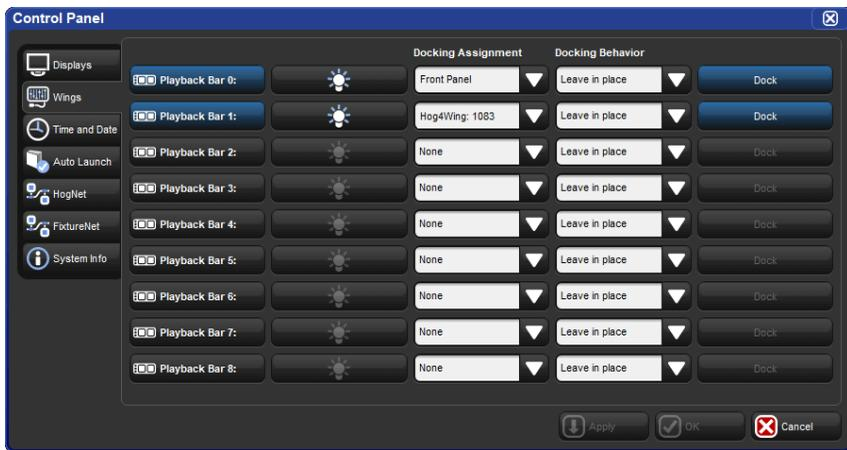
Figure 3.8. Wings pane of the Control Panel with active front panel and wing docking assignments
