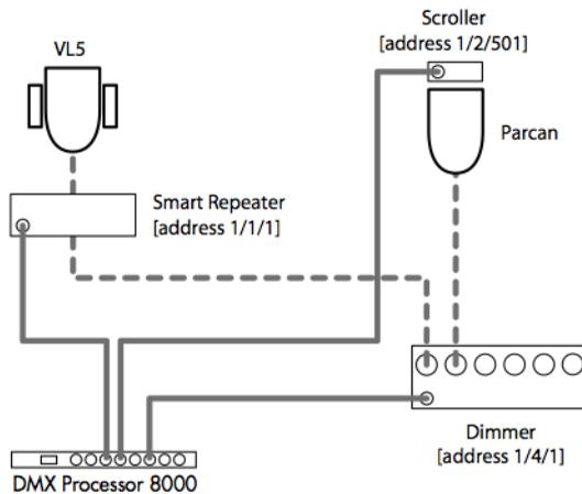
Figure 5.3. Examples of Fixtures requiring Multiple Patch Points
