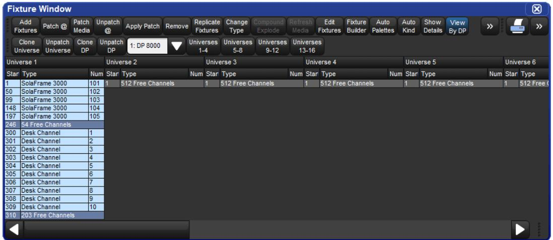
Figure 5.2. The View by DP view of the Fixture window
