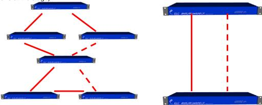
On the front panel there is a red LED called Allert, this will be on if a loop is broken.
