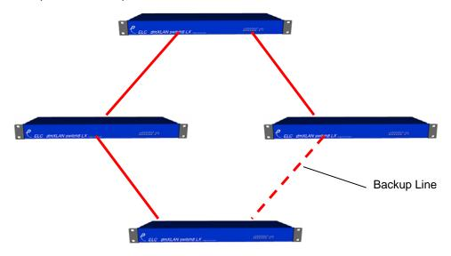
When using standard Ethernet switches, a loop of switches will bring the network down. With the switch8LX ports programmed to loop, the "Backup Line" is detected and automatically disabled. If then during operation (the show) one of the working lines gets broken (or disconnected) all the switch8LX's will then reroute the signal using the backup line, this within 30 to 50 mSec.
