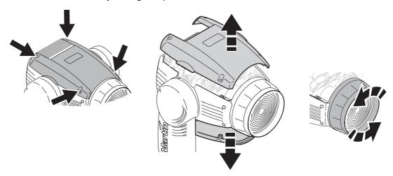
Figure 10: Releasing top and bottom covers and removing front lens
