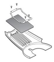
Figure 12: Air filter replacement
