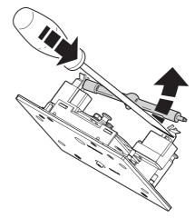
Figure 2: Lamp removal
