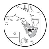
Figure 11: Main module locking levers
