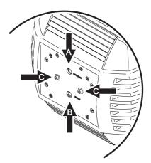
Figure 5: Lamp adjustment screws
