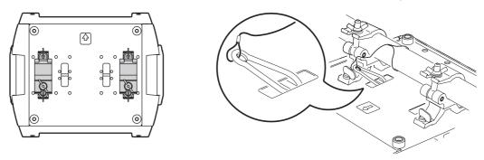
Figure 6: Clamp bracket positions and safety wire attachment point
